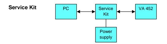
The diagram above shows the connection when using the optional service kit (0554 2005). Please ensure that also in this case the power supply of either VA 452 or of the service kit is connected (USB port is not supplying enough power).
