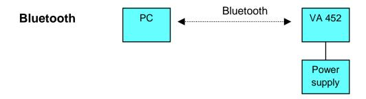
Bluetooth provides a convenient way of configuring the sensor without the hazel of cable connections. VA 452 needs to be powered up. Ensure that the distance between VA 452 and PC is no more that 5 meter and the PC Bluetooth antenna should point roughly in the direction of the display (front part). Please follow the instruction in the service software and the help file.
