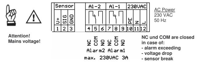
DS 51 has one analogue sensor input for connection of sensors with 0/4...20 mA signal. The sensor input is configurated on our premises (according to the customers specification in the order).
